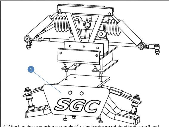
4. Attach main suspension assembly #1 using hardware retained from step 3 and tighten. A floor jack is recommended to hold the suspension assembly in place while you get the bolts started.
