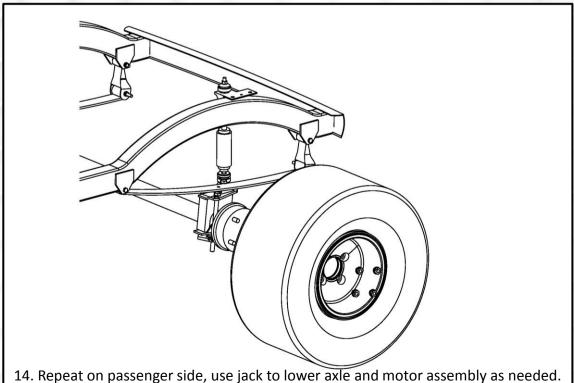
14. Repeat on passenger side, use jack to lower axle and motor assembly as needed. Once complete, install wheels, lower cart and proceed with alignment on next page.
