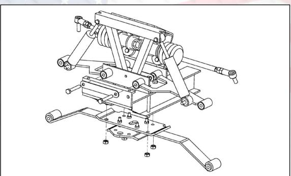
3. Remove the four factory A-arm bolts and nuts. Remove factory A-arms, do not retain. Remove the four bolts and washers to detach factory suspension assembly and retain hardware. Factory suspension assembly will not be used.
