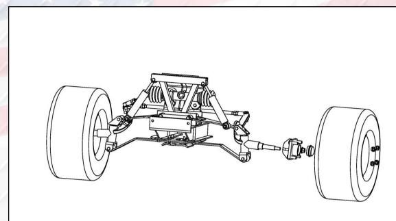
1. Remove front bumper and retain. Remove front wheels. Remove dust cap, cotter pin, spindle nut and wheel hub. Retain hub and hardware.
