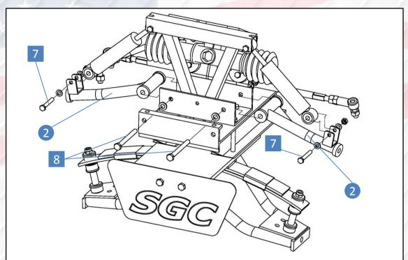
5. Install upper arm #2 on the cart using supplied hardware #8. Install lower end of factory shock on the upper arm using hardware #7.
