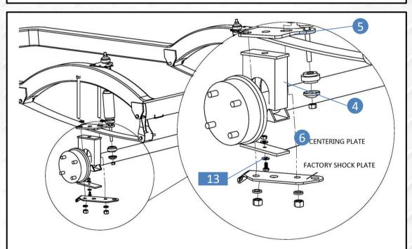
12. Place rear lift block #4 on the axle and under leaf spring. Ensure that top of lift block angles down toward the front of cart. Place rear shock plate#5 over leaf spring and attach shock to it. Attach hardware #13 on centering plate #6 then attach centering plate to factory shock plate. The bolt head and nut will fit into the center hole of the spring perch and factory lower bracket to aid in alignment of the riser and mounting plates.
