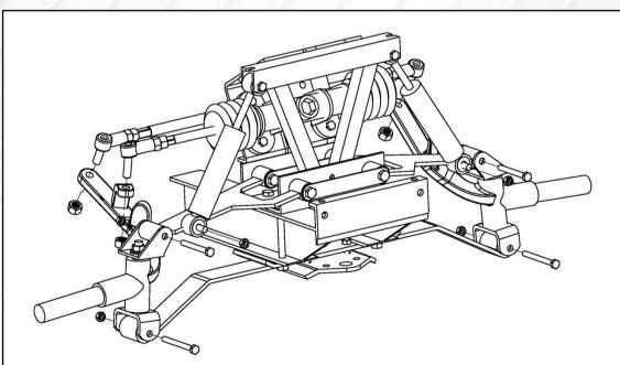
2. Remove lower shock mounting bolt and nut on driver and passenger side. Shock does not need to be completely removed, only the lower bolt so the shock can be pushed up and out of the way. Remove spindles from leaf spring and drag link and tie rod end. Retain Hardware.
