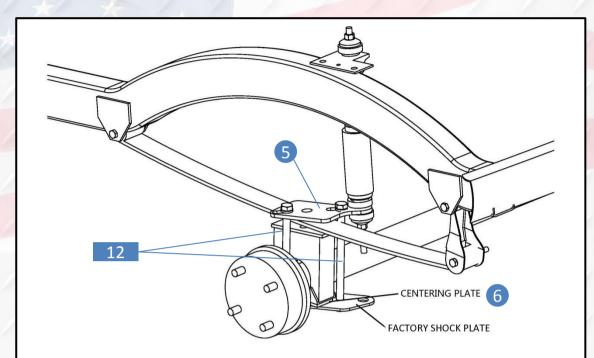
13. Route bolt from supplied hardware #12 through rear shock plate #5, rear lift block and factory shock plate. Using socket to tighten these four bolts evenly to ensure proper alignment.
