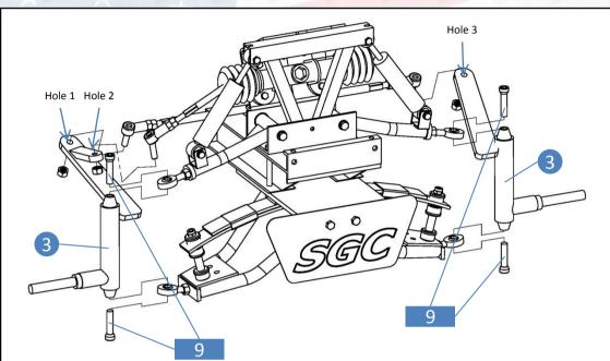
7. Attach spindles #3 between two heim joints using hardware #9 and tighten. Attach steering linkage to upper portion of spindles on both sides using hardware retained and tighten. Attach drag link using retained hardware and tighten.
