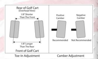
IMPORTANT: Both Camber and Toe must be adjusted on this model.
