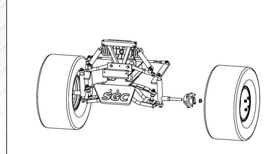
8. Reattach hub and dust cap using hardware retained from step 1. Install new front wheels and bumper using hardware retained from step 1. Do not attempt to align cart until installation is complete.
