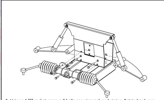
5. Using a 1/2" socket remove 3 bolts securing rack and pinion. Retain hardware. You will not completely remove rack and pinion. This step is to gain access to upper A-arm bolts. Using a 1/2" socket remove factory A-arms. Retain hardware.
