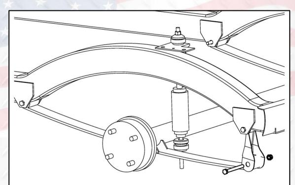
12. Using a 10mm socket and 13mm wrench remove hardware from rear leaf spring mount and front leaf spring mount. Retain hardware.
