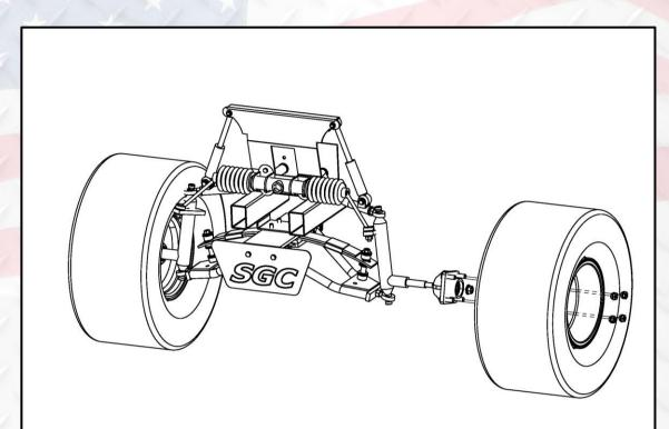
9. Reattach hub using hardware retained from step 2. Reinstall bumper . Install new wheels and lower cart.
