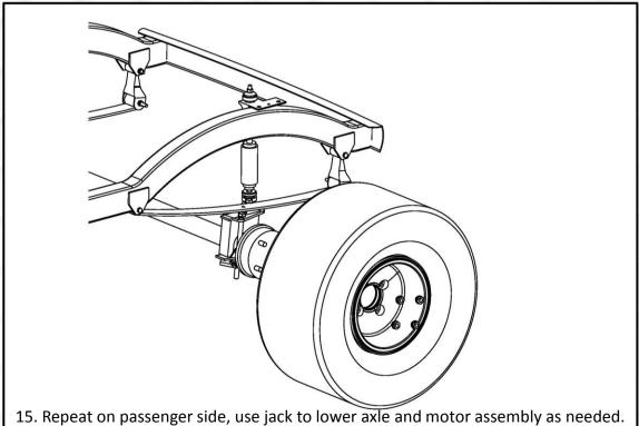
15. Repeat on passenger side, use jack to lower axle and motor assembly as needed. Once complete, install wheels, lower cart and proceed with alignment on next page.
