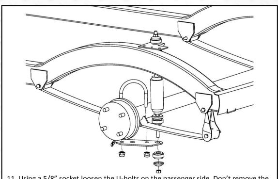
11. Using a 5/8" socket loosen the U-bolts on the passenger side. Don't remove the U-bolts. It's important to do one side at a time to avoid motor roll. Loosening but not removing the U-bolts will make this easier.
