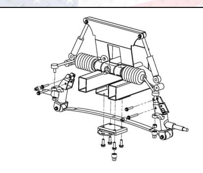
3. Using a 1/2" socket remove bolt from shock and discard. Push shock up and out of the way. Remove and retain the cotter pin from tie rod end, using an 18mm socket and 11/16" wrench. Remove nut from tie rod.
