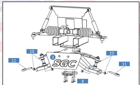
7. Using spring plate from step 4. Attach new main suspension assembly #3. Use supplied #8 hex bolts and washers to secure to cart. Before attaching spindles, install and adjust heim joints so there is approximately 1/4" of thread showing.
