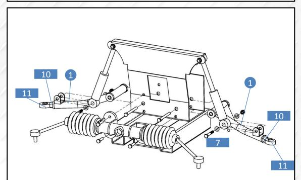
6. Install supplied upper a-arm #1 to cart with hardware from last step. Install heim joint #11 and nut #10 to upper a-arm. Install factory shock to upper a-arm with supplied hardware#7 5/16-2 bolt washer and nut.
