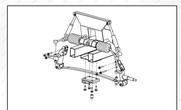
4. Using 1/2" socket remove factory spindle. Using a 1/2" socket remove sping plate and leaf spring. Retain spring plate, discard harware and leaf spring.
