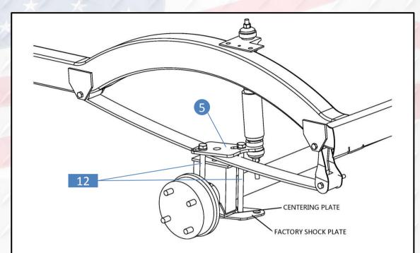
14. Route supplied #12 bolts M12\*180 through rear shock plate#5, rear lift block and factory shock plate. Using socket to tighten these four bolts evenly to ensure proper alignment.
