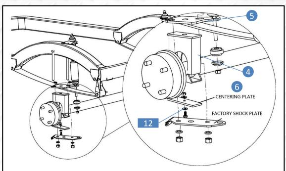
13. Place rear lift block #4 on the axle and under leaf spring. Ensure that top of lift block angles down toward the front of cart. Place rear shock plate#5 over leaf spring and attach shock to it. Attach hardware #13 on centering plate #6 then attach centering plate to factory shock plate. The bolt head and nut will fit into the center hole of the spring perch and factory shock plate to aid in alignment of the riser and mounting plates.
