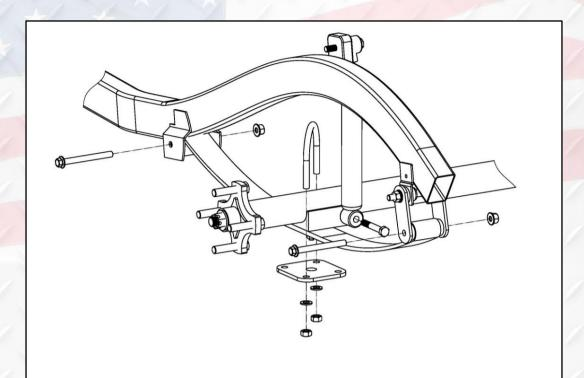
11. Using 15mm socket remove drive side shock, factory U-bolt and spring, spring retaining plate. Retain spring and hardware.
