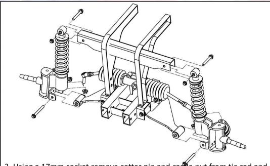
3. Using a 17mm socket remove cotter pin and castle nut from tie rod and remove the tie rod from the spindle. Retain hardware. Using a 15mm socket and wrench remove hardware from top of shock and from the lower control arm.
