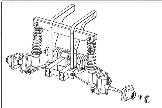
2. Using a 15/16 socket remove cotter pin and castle nut from spindle. Remove hub. Retain hub and hardware.
