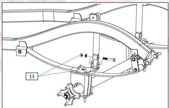
13. Route supplied U-bolt #13 down through the top of the rear shock plate to the bottom factory Bracket. Be sure that all alignment bolts are in correct position to keep axle straight. Using a 17mm socket tighten U-bolt evenly to ensure proper alignment. Attach shock to rear shock plate #7 using factory bolt, washers and supplied lock nut from #13.
