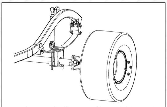
14. Use jack to lower axle and motor assembly as needed. Once complete, Install new wheels, lower cart and proceed with alighment.
