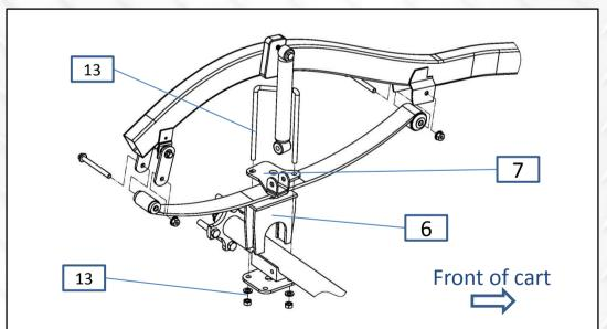
12. Reinstall factory leaf spring above the axle and install rear lift block #6 under the leaf spring as shown. Check spring bushings for rust and wear. Replace if necessary. Place rear shock plate #7 on the spring.
