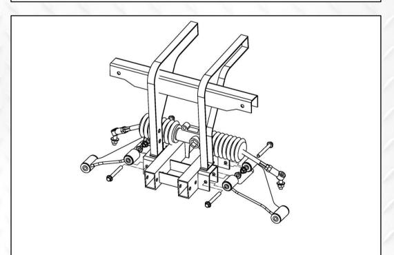
4. Remove lower control arm from the cart. Retain it and the hardware.
