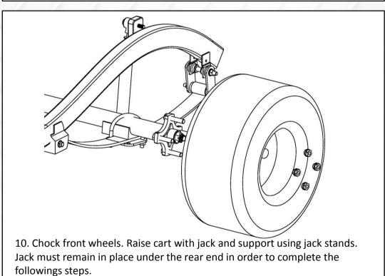
**Caution**: The jack will be used to support the entire rear end assembly (axle and motor) for a short time while the leaf springs are moved into their new position above the axle. In order to prevent damage to the axle and motor assembly, jack must remain in place, but only apply enough pressure to keep the rear end assembly from falling.
