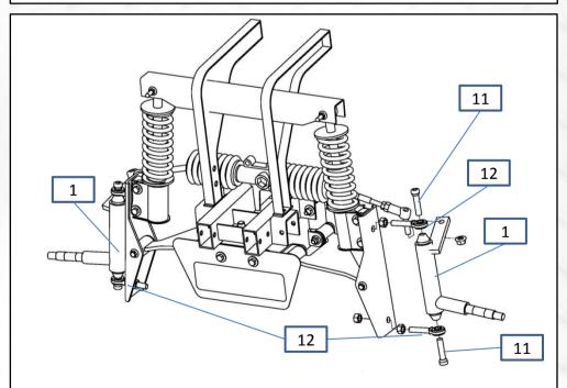
8. Attach heim joints #12 to spindle bracket using nuts #12. (One nut on top, two nuts each side on bottom). Attach supplied spindle #1 to spindle bracket #5 using hardware #11.
