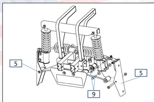
7. Attach spindle bracket #5 to shock absorber #3 using hardware #9. Attach spindle bracket #5 to lower control arm using factory hardware.
