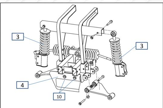
6. Reattach lower control arm to cart using factory hardware. Attach top of supplied shock absorber #3 to cart using factory hardware. Then attach SGC plate #4 to main frame #2 using hardware #10.
