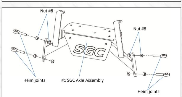
7. Install heim joints on SGC Axle Assembly #1. Use two nuts each from hardware #8. The camber could be adjusted by repositioning the nuts. Recommeded nut position for most carts is as shown in below picture. **Don't tighten the nuts until bolts and nuts are tightened in Step 10.**
