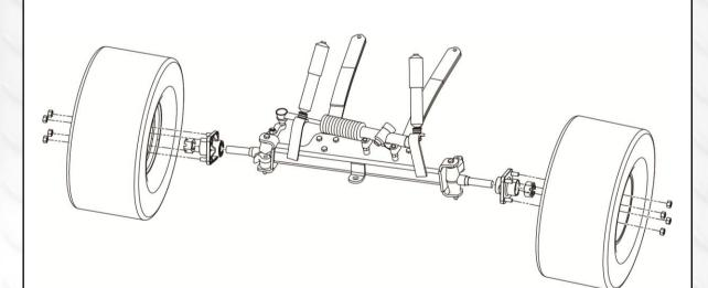
1. Engage parking brake and chock rear wheels. Raise Golf Cart with lift and use jack stands. Remove front tires, then remove cotter pin, castle nut, and hub. Retain hardware.
