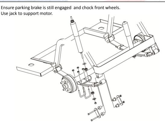
14. Unbolt the rear leaf springs from under the rear end. Save the front and rear leaf spring bolts for reinstallation of the leaf springs. Using the car jack lower the rear end of the cart.
