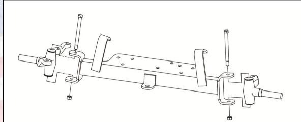
6. Remove spindles from drop axle.
