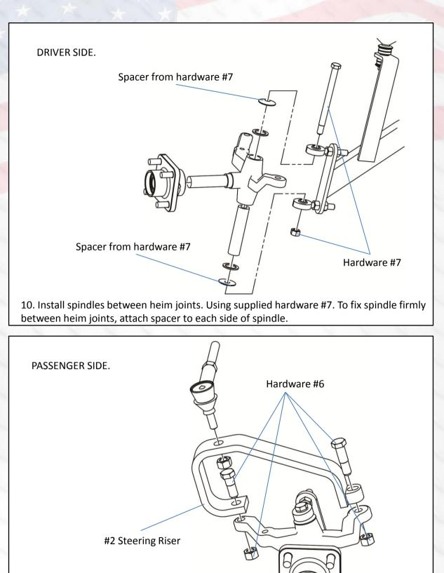
11. Install steering riser #2 on spindle using supplied hardware #6. Install rack ball joint on steering riser using retained hardware.
