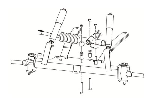
4. Remove three bolts from rack and pinion. Retain Hardware.
