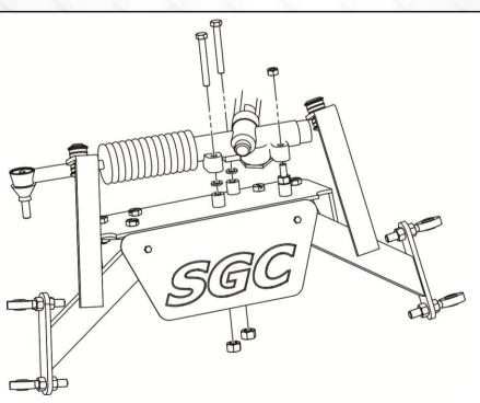
9. Install front bolt for rack and pinion. IMPORTANT: For ease of installation, frontmost bolt for rack and pinion must be installed before spring plates are reattached.
