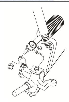
2. Remove cotter pin from castle nut. Remove castle nut from ball joint and separate ball joint from spindle. and retain.
