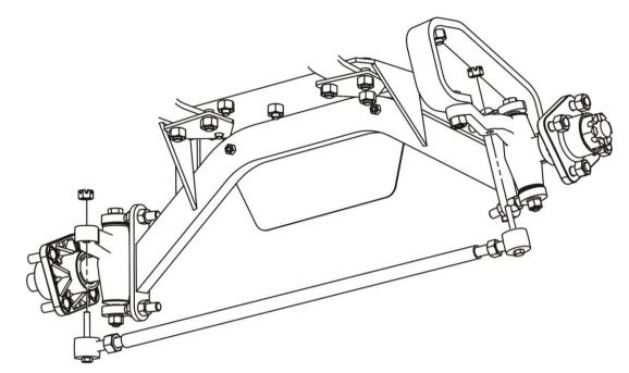
12. Install tie rod to spindles using retained hardware. Reinstall hubs. NOTE: SOME E-Z-GO MODEL CARTS COME STOCK WITH A TIE ROD LONG ENOUGH! IF THE STOCK TIE ROD JOINTS DO NOT HAVE GREASE FITTINGS FROM WHEEL TO WHEEL YOU WILL NEED TO INSTALL THE TIE ROD IN THIS KIT.
