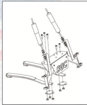
8. Install SGC Axle Assembly to leaf spring and spring retaining plate with factory hardware.
