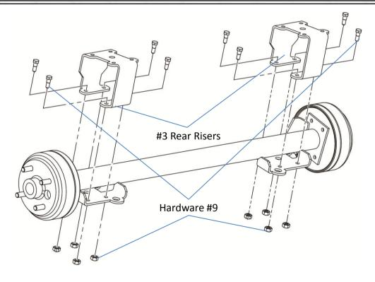
15. Install Rear Riser #3 on top of the axle using supplied hardware #9.
