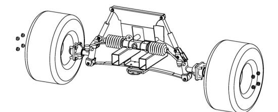
1. Remove lug nuts when cart on ground. Then raise the cart with jack stands under the frame. Remove wheel from the hub. Detach front bumper and retain hardware.
