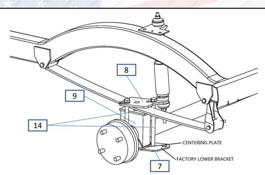
14. Route supplied bolts M12\*180 through shock plate #8, rear lift block #9 and factory lower bracket making sure centering plate #7 fits properly. Using socket to tighten these four bolts evenly to ensure proper alignment.
