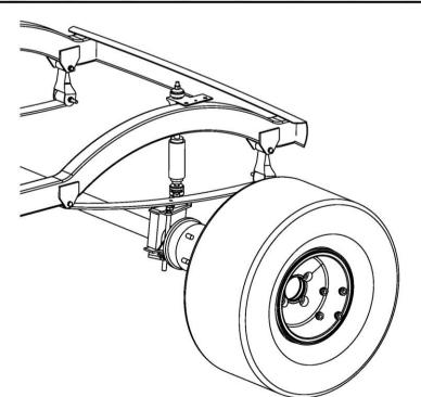
15. Repeat on passenger side, use jack to lower axle and motor assembly as needed. Once complete, install wheels, lower cart and proceed with alignment on next page.
