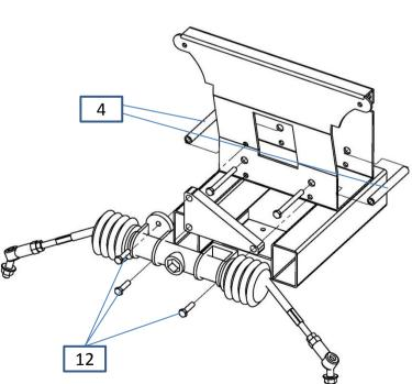
Reinstall rack and pinion and supplied spacer to cart frame using supplied hardware #12.
