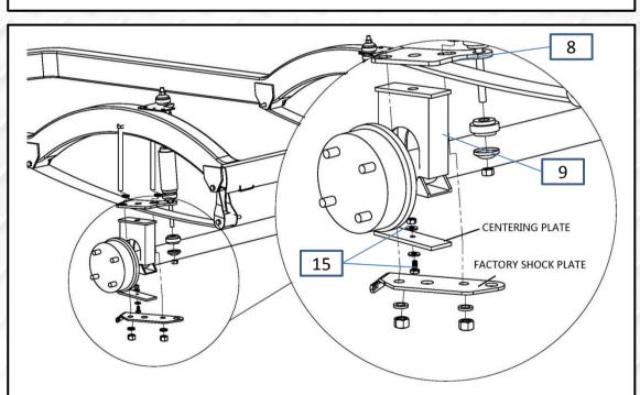
13. Place rear lift block #9 on the axle and under leaf spring. Ensure that top of lift block angles down toward the front of cart. Place rear shock plate #8 over leaf spring and attach shock to it. Attach hardware #15 on centering plate #6 then attach centering plate #7 to factory shock plate. The bolt head and nut will fit into the center hole of the spring perch and factory shock plate to aid in alignment of the riser and mounting plates.
