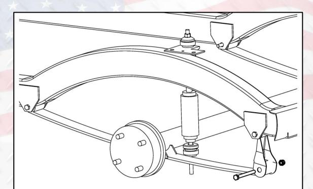
14. Using a 10mm socket and 13mm wrench remove hardware from rear leaf spring mount and front leaf spring mount. Retain hardware.
