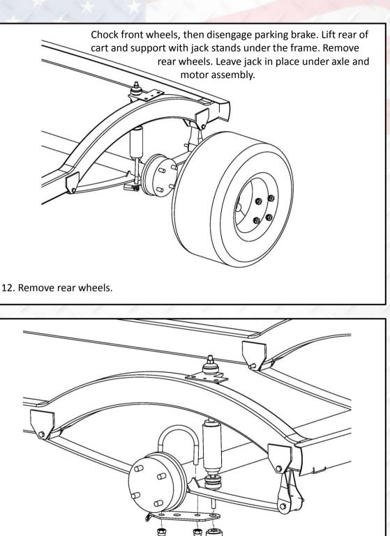
13. Using a 5/8" socket loosen the U-bolts on the passenger side. Don't remove the U-bolts. It's important to do one side at a time to avoid motor roll. Loosening but not removing the U-bolts will make this easier.
