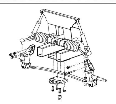
4. Using 1/2'' socket remove factory spindle. Using a 1/2'' socket remove spring plate and leaf spring.
