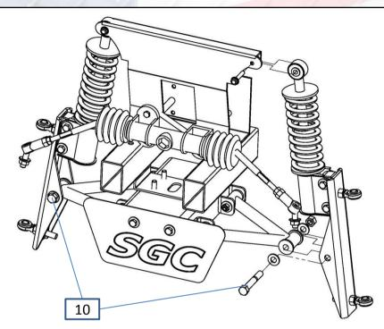
9. Attach spindle bracket #2 to upper a-arm from main suspension frame using supplied hardware #10 (detached in step 7). Attach top of shock absorber #5 to cart frame using factory hardware from step3.
