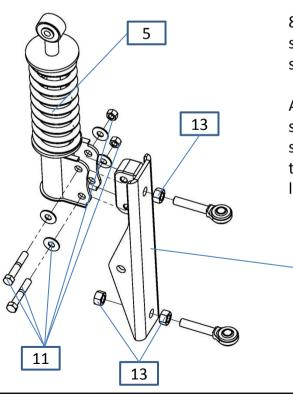
8. Attach shock absorber #5 to spindle bracket #2 using supplied hardware #11.
