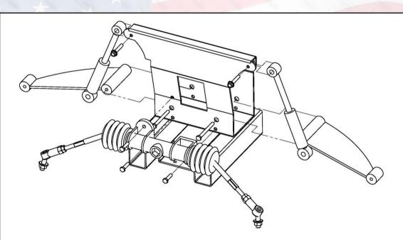
5. Remove rack and pinion, upper a-arm and factory shock absorber.
