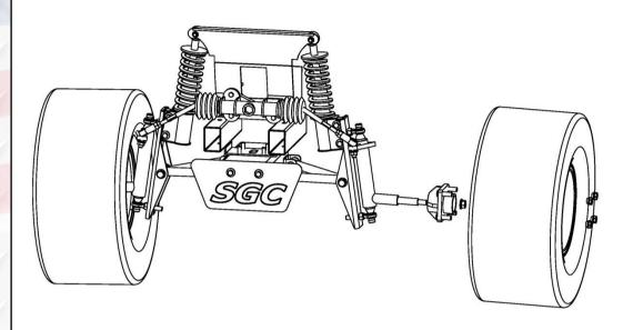
11. Reinstall hubs and install new large wheels.
