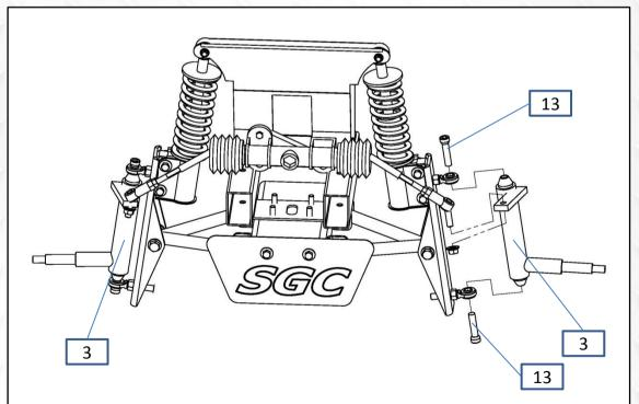
10. Install supplied spindle #3 on heim joint using supplied egg neck bolt #13. Attach tie-rod end to spindle using factory hardware.
