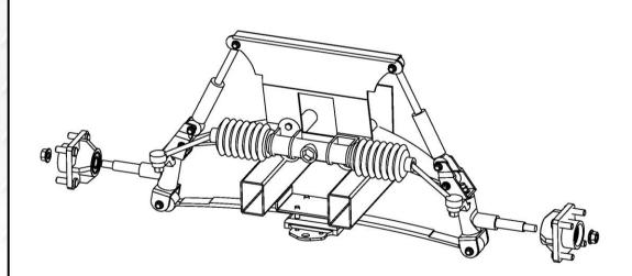
2. Using a 21mm socket remove and retain hub and flange nut. Repeat on passenger side.
