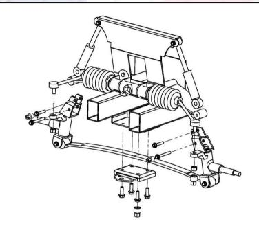
3. Using a 1/2'' socket remove bolt from shock and retain. Push shock up and out of the way. Remove and retain the cotter pin from tie rod end, using an 18mm socket and 11/16'' wrench. Remove nut from tie rod and retain.
