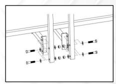
2. Install grab bar to mounting bracket using 4 supplied 1/4-1 3/4 bolts, washers and nuts.
