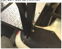
•Install rear roof supports using (4) bolts / nuts / washers of E-5 on arm tube.
