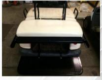
3. Install seat cushion on cargo bed using (6) self-drill screws of E-3.
