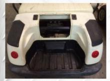
1. Take canopy / rear roof supports / main bracket / basket / engine cover off the cart, keep (4) factory bolts took off from main bracket for future use.
