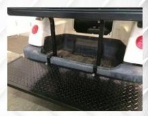
6. Attach foot plate to vertical supports using (2) bolts / nuts / washers of E-4.
