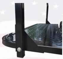
7. Attach arm tube to cargo bed / foot plate using hardware E-1. LONGER ONES ON FOOTPLATE SIDE. Install triangle brackets between arm tube and footplate.
