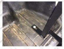
4. Install vertical supports using (2) factory bolts on bag well liner.
