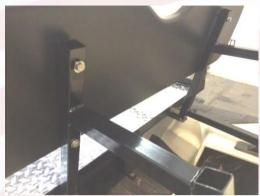
8. Install rear seat back cushion using (4) bolts of E-3.
