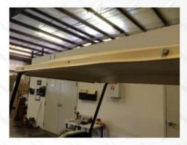
•Install canopy on rear roof supports using (2) bolts / nuts / washers of E-6. Using factory bolts / nuts / washers install on front holes.
