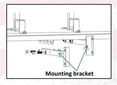
1. Install mounting bracket to footplate using 4 supplied 1/4-1 3/4 bolts, washers and nuts.
