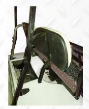
Step 9: Install front back cushion using factory hardware. Install rear seat back cushion on the main bracket using hardware D-3.
