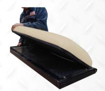
Step 2: Install seat cushion on flipping cargo bed use 6 self-drill screws from hardware D-3.
