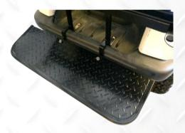
Step 7: Install foot plate on vertical supports using hardware D-4.
