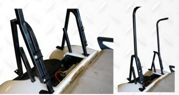
Step 4: Install two rear roof supports on main brackets using hardware D-5
