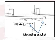
Install mounting bracket to footplate using 4 supplied
