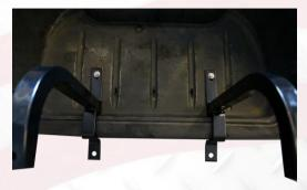
Step 5: Install vertical supports on cart's bagwell area using hardware D-6. You have to enlarge the mounting hole using supplied drill bit. Reattach the access panel cover back to cart using original factory fasteners.
