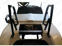
Step 3: Install main bracket on cart using original factory hardware. Tight the bolts from inside the cart.
