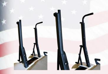
Step 4: Install plastic water drain rear roof support bars on steel rear roof support bars using original factory fasteners.
