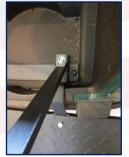
5. Install two vertical supports on foot plate bracket using hardware R-3.
