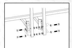
2. Install grab bar to mountingbracket using 4 supplied1/4-1 3/4 bolts, washers and nuts.
