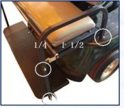
8. Install seat cushion on flipping cargo bed using 6 self-screws from hardware R-4. Then install flipping cargo bed on vertical supports and back support angles using hardware R-2. Install arm tube on flipping cargo bed and foot plate using hardware R-1 (longer bolts on foot plate).
