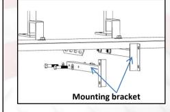
Install mounting bracket to footplate using 4 supplied
