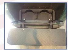
6. Install foot plate bracket with vertical supports assembly on cart's bagwell area using existing factory hardware. Tips: Install vertical supports first.
