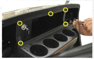
8. Using a phillips head screw driver, remove the 5 screws on the dash board and retain hardware.
