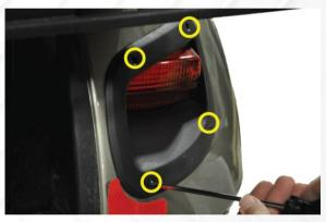
6. Place tail light into the rear of the vehicle. Insert four self tapping screws into tail light using supplied hardware.\*Repeat process on other side.
