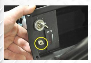
11. Reattach Push/Pull switch to harness. Remove small washer and retain. Feed threaded end of switch through the dash where the hole was drilled.
