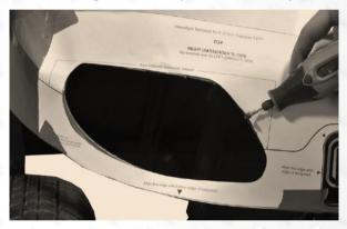
1. Place template on front of the cart. Be sure to use alignment references for proper placement. Tape along the ridges in the cowl. Mark along the inside with a marking pen. Drill pilot hole on the inside of the template line. Cut out the shape of the headlight. Use the cutting tool to remove the excess trim. \*Flip template over repeat process on the other side.
