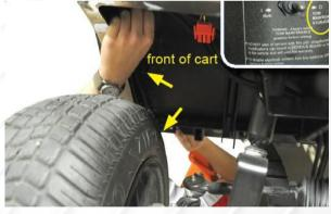
3. \*Make sure cart is in TOW mode. Lift front of the cart and place jack stands to support. Feed front harness down through the front of the battery comparment. Run long tail light wire under the seat and over the tire well on the passenger's side. Run short tail light wire under the seat and over the tire well on the driver's side Red plugs should be aligned to passenger side, white plugs for driver's side.
