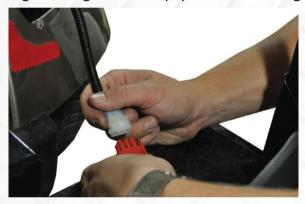
5. Feed the tail light harness through the back of the cart. Attach rear tail light wire harness as shown. Secure wire with ties.
