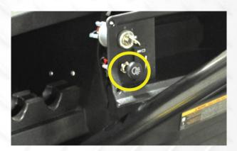
12. Attach the nut to tighten the switch. Reattach Push/Pull knob. Using retained hardware to reattach dashboard.
