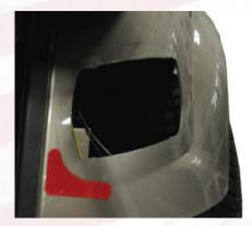
4. Align Tail Light template to the body contour as shown. Be sure to use alignment references for proper placement. Use a marking pen to trace the inside line. \*Flip template over to use on other side. Next drill a pilot hole so you will have a starting point and then begin cutting. \*Use sandpaper to smooth edge.
