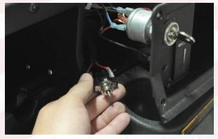
10. Feed the Push/Pull switch wire through the dashboard.
