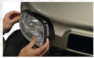
2. Use sandpaper to smooth out any rough edges. Mount headlight through the cutout. Push top half in first as shown.
