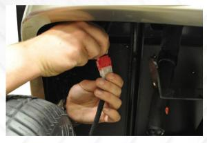
7. Remove the push/pull switch from harness. Run the wire harness through the holes under the frame to secure the harness. Use the zip ties provided. Attach headlight to wire harness as shown. Secure excess wire with zip ties.
